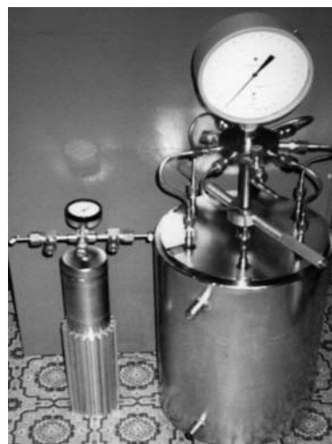
Fig.5. A general view of two types of the hydrogen accumulators.
