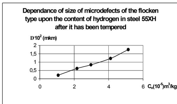
structure of steel of the 55XH type it was obtained the dependence of sizes of flocken type defects which is represented in Fig.3 upon the content of hydrogen after the tempering of steel.
