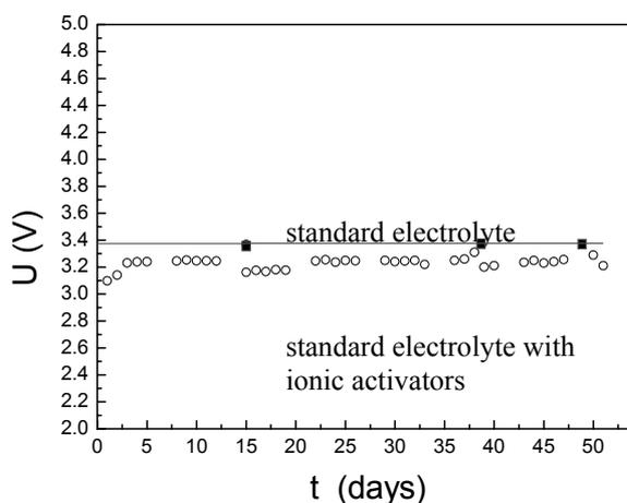
Figure 2. Long term run electrolysis: Illustration of the ionic activator effects.
