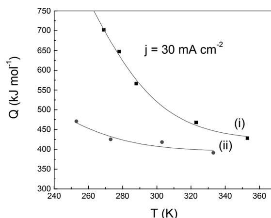
Figure 1. Energy consumption per one mole of hydrogen evolved as a function of temperature for two electrolytic cells.
