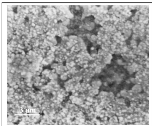
Figure 2. SEM microphotography of the Ni cathode, which was used for electrolysis with ionic activator (Co-Mo combination).
